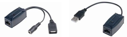
The UE01 USB extender design for extends USB device with full speed up to 70 meters or low speed up to 300 meters from the location of your computer over CAT5/5e/6 UTP cable. It could eliminate the 5 meters distance limitation of USB. It is optimized for applications where two devices, such as the keyboard and mouse, must be operated remotely.
